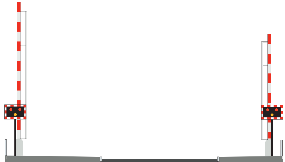
Standard wigwag lighting and barriers
